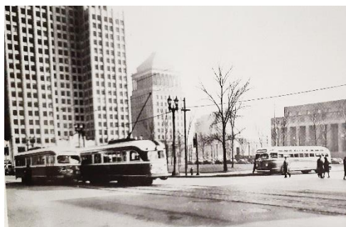
Two cars from St. Louis’ initial order pass on Olive at 14 th Street in 1940. These were the first production all-electrics. Note the 36-passenger Yellow Coach to the right and the Soldiers Memorial behind it.
